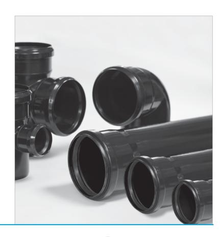
EasyFONO is the soundproof system for wastewater consisting of push-fit pipes, fittings and accessories, with a wide range of diameters DN32 to DN160, for pipes, and from DN32 to DN110 for fittings. Pipes and fittings are made of mix of polypropylene with mineral fillers to ensure a good soundproofing performance.
